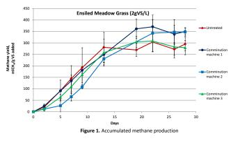
were loaded with the same grass amount and subsequently, their effect on the biomethanation process was examined. Concerning the second test, the effect of different grass load was examined only in the most promising comminution machine, according to the results obtained from the first BMP test.
