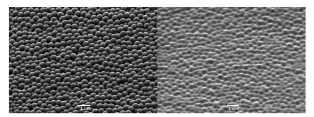
Figure 1: A nanostructured nickel tool insert (left) and a polypropylene replication (right) made by injection moulding without applying induction heating to the tool. It is obvious that replication is not as sharp as the tool, but this can be dramatically improved by introduction local heating of the tool insert.
