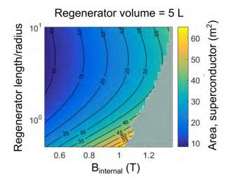
Figure 1: The area of the superconducting tape needed to produce a desired internal magnetic field for a given aspect ratio of the regenerator cylinder.
