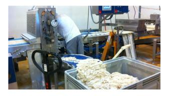
Figure: 1: Waste material due to height differences on the belt (fixed with the fellow fork truck)
