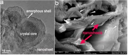
(a) Crystalline@amorphous core/shell Co<sub>3</sub>O<sub>4</sub> nanoparticles decorated ultrathin Co<sub>3</sub>O<sub>4</sub> nanosheets, (b) NiO nanowires (the white arrows) decorated NiO nanosheets
