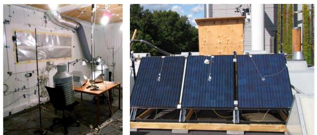
Figures. Experimental chamber with PCM radiant ceiling (left) and PV/T panels (right).
