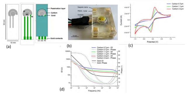
Figure 1: Top view of the microelectrodes composed of a circular carbon working electrode (WE), surrounded by a carbon counter electrode (CE), gold reference (RE), and passivation layer (SU8) (a), selfaligning magnetic clamping system for electrochemical analysis (b), CV spectra in ferri-ferrocyanide (c) and impedance spectra in PBS (d) of the optimized electrode with long gold leads and increased carbon thickness
