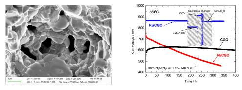
Figure (left): Porous ceramic electrode with impregnated Ba-oxide, (right): durability test of a full ceramic SOFC anode.
