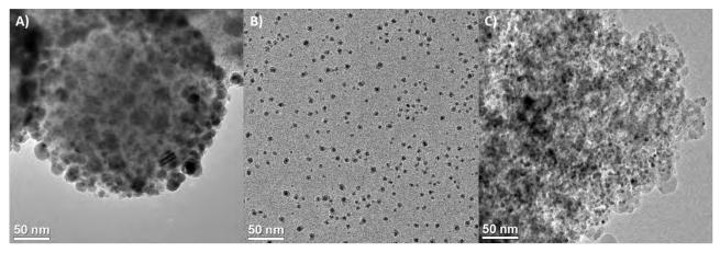
TEM micrographs of NiGa NPs supported on A) 200 nm SiO<sub>2</sub> spheres, B) SiO<sub>2</sub> membranes and C) High surface area SiO<sub>2</sub> support.
