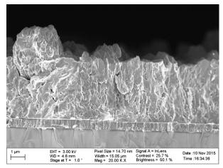
Fig. 1: SEM cross-sectional image of a CZTS layer identical to the one used in a 0.2 % efficient solar cell. The CZTS layer (4-5  $\mu$ m thick) is deposited on a 500 nm layer of Mo that has been sputtered on soda lime glass.
