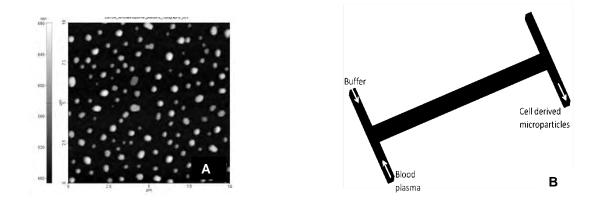
Figure 1:. A/ AFM topography image of microparticles derived from HUV-EC-C after undergoing apoptosis for 24 hours. B/ Scheme of the device for isolation of MPs
