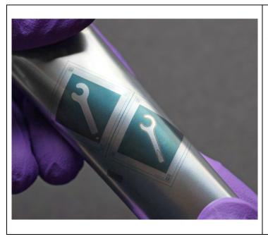
Flexible plastic foil with embedded plasmonic color meta-surface decoration. The color appears from a thin film of aluminium deposited on top of a nanotextured surface.
