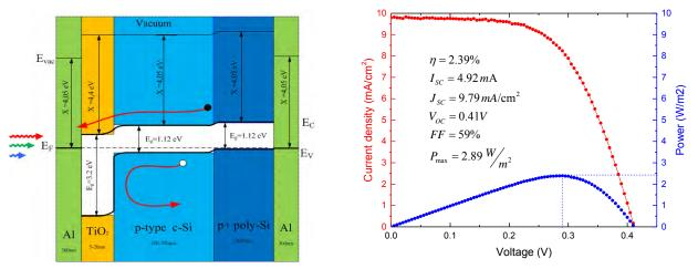
Figure 1: Energy band diagram of TiO2-Si-poly Si structure (left), current-voltage and power –voltage characteristics (right)
