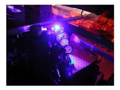
Figure 1. The recently developed 3D polychromic stereolithography printer at DTU Nanotech can expose with multiple wavelengths, here 365 nm and 450 nm, at <15 μm pixel size to freely combine multiple materials within a printed object.
