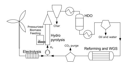
**Figure 1** Proposed process diagram including catalytic hydropyrolysis, char separation, temperature adjustment, deep HDO, liquid separation, pyrolysis gas reforming and water gas shift (WGS). Additional hydrogen may be obtained from water electrolysis.
