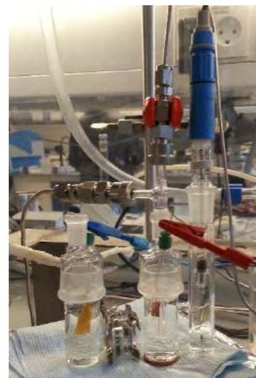
Figure 1: Liquid cell for measurement of CO<sub>2</sub> reduction products. Shown here with a Cu sheet electrode as electrocatalyst.
