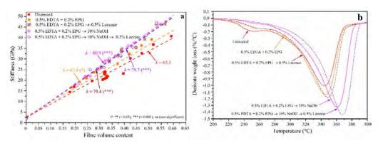
**Fig.1.** (a) Stiffness of composites reinforced with differently treated fibers and (b) Thermogravimetric analysis for derivatives of weight (%) vs. temperature (°C) of untreated and differently treated hemp fibres.
