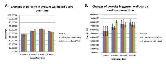
Figure 1. Water and fungal growth influence on porosity of core (A) and cardboard (B) from gypsum wallboard.
