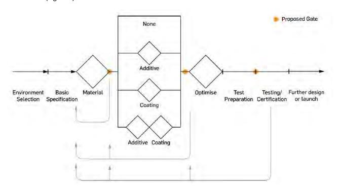
Figure 1: Guidelines for Design for Biodegradability
