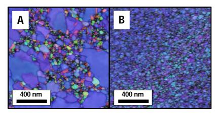
Figure 1 – TKD images of 20nm Au (A) and 2nm Ti + 20nm Au (B) samples. Au sample shows high grain size dispersion. We observe a general decrease in grain size and dispersion for the sample with Ti adhesion layer.
