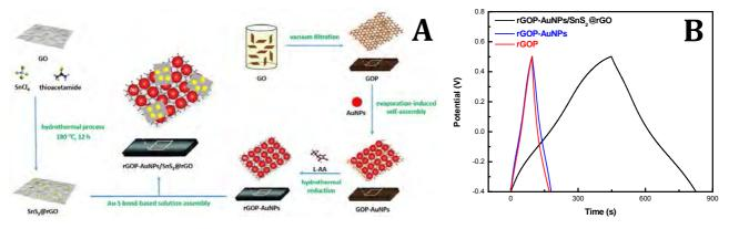
Fig.1 (A) Schematic for the fabrication process of rGOP-AuNPs/SnS<sub>2</sub>@rGO paper electrodes. (B) Charge-discharge curves of rGOP-AuNPs/SnS<sub>2</sub>@rGO, rGOP-AuNPs and rGOP at 0.5 A·g<sup>-1</sup>.
