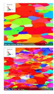
Figure 1: Orientation maps before and after cycling for 5000 cycles obtained by ESBD showing developing subgrain structures
