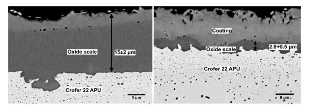
**Figure 1**: SEM cross sectional micrographs of samples oxidized 2000 h at 900 °C in air. Left: uncoated Crofer 22 APU alloy. Right: Crofer 22 APU coated with MnCo₂O₄.
