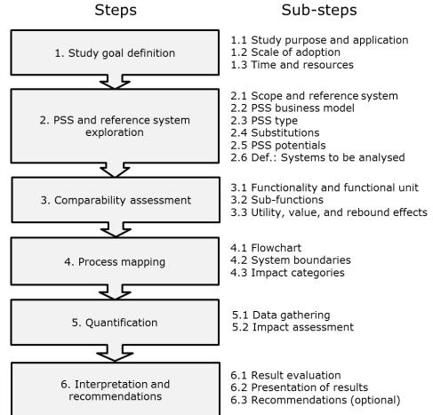
Figure 1: Guideline steps and sub-steps for PSS environmental evaluation
