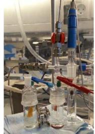
Figure 1: Liquid cell for measurement of CO<sub>2</sub> reduction products. Shown here with a Cu sheet electrode as electrocatalyst.
