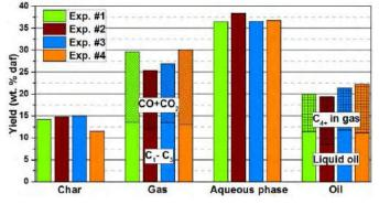
**Figure 1:** Photograph of the recovered liquids from Exp. #4, oil is top phase. Yields of char,  $C_1$ - $C_3$  hydrocarbons, CO +  $C_2$ , condensed aqueous phase and condensed oil with potentially condensed oil ( $C_{4+}$ ) in gas phase on dry, ash free basis for Exp. #1 to #4. The mass balance sum to 100, 98, 100 and 101 % respectively.
