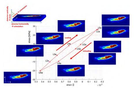
Figure 2: Azimuthal maps acquired during a single tension-compression load cycle at APS 1-ID-E using High Resolution Reciprocal Space Mapping. Azimuthal maps are projections of the intensity distribution along the scattering vector representing the internal structure and orientation distribution within individual grains.
