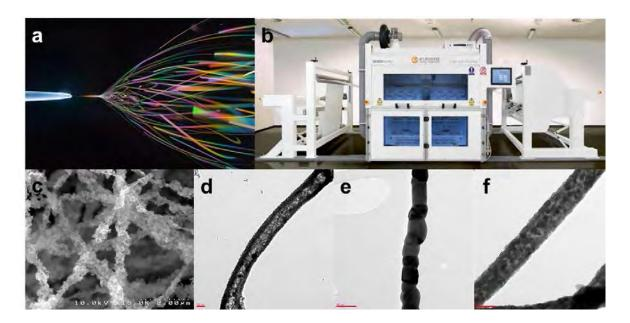
**Figure 1.** a) Electrospinning process; b) Industrial-scale electrospinning equipment (Elmarco); c) Pt-C/Nafion nanofiber electrodes for PEMFCs; d) metal oxide nanotubes; e) metal oxide nano-pearl string; f) metal oxide nanofiber.
